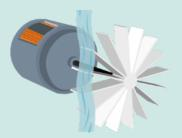
Electricity is made using a generator. A simple generator can be made by spinning a magnet around inside a coil of wire.
